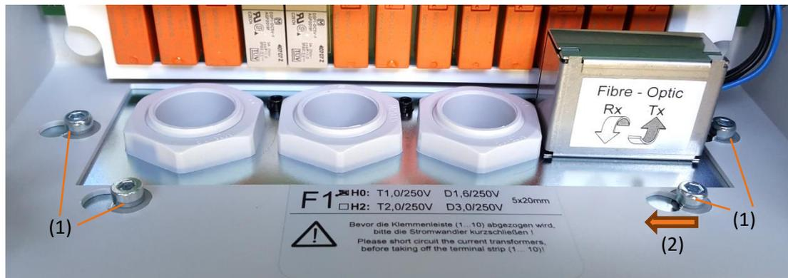
*Flange plate with fibre optic connections*
