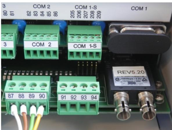
*Fibre optical connection (1 x Ethernet-ST, XW93) at Level II; REG-DA Com ports at Level III*
