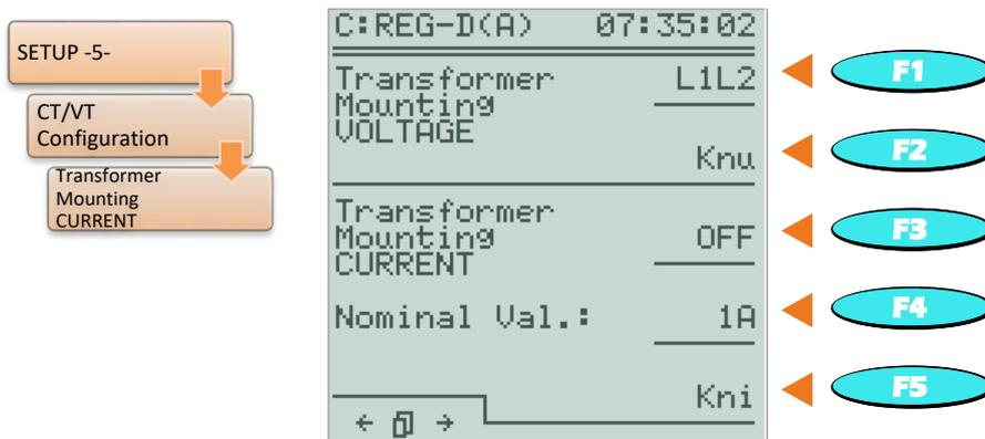
To use the REG-DA, it is not necessary to assign the current measurement terminals a specific location in the grid in terms of hardware (e.g. I1). Regardless of which phase the current is measured in, the regulator determines the correct angular relationship when the actual connection is set in the CT/VT Configuration menu.
