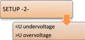
The following figure gives an overview of the configurable voltage limits of the REG-DA. Starting from the setpoint, the permissible setpoint deviation forms a tolerance band (positive and negative bandwidth), in which there is no automatic voltage regulation.
