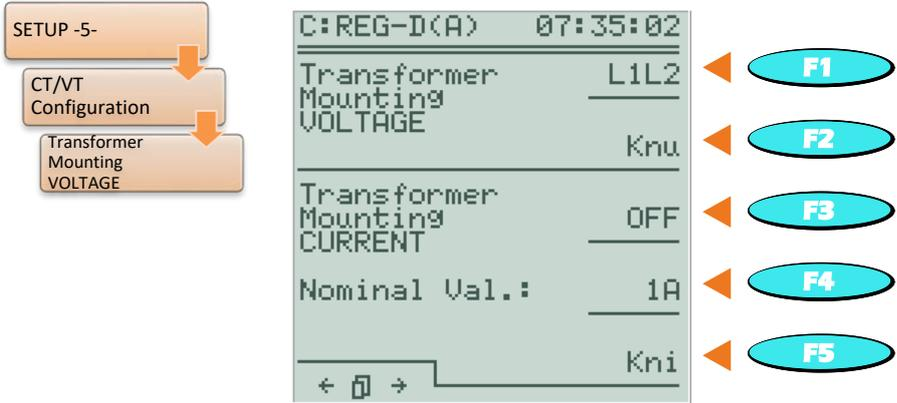
To use the REG-DA hardware it is not necessary to assign voltage measurement connections to a particular position in the network (e.g. U12). Regardless of which external conductors the voltage is measured between, the regulator determines the correct angular relationship when the actual connection is set in the CT/VT Configuration menu.
