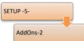
To also show the present current measurement next to the present voltage reading on the regulator basic display, the current display can be activated in the menu “functions”.
