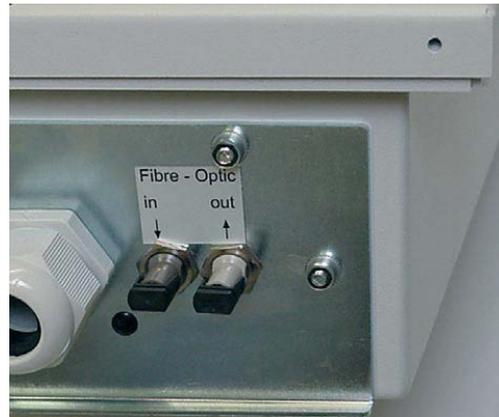
*Fibre optical connection (ST-connector, V17, V19)*
