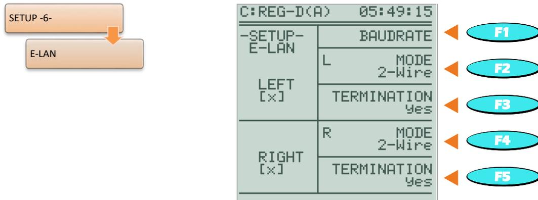
Each regulator provides two complete E-LAN interfaces.
