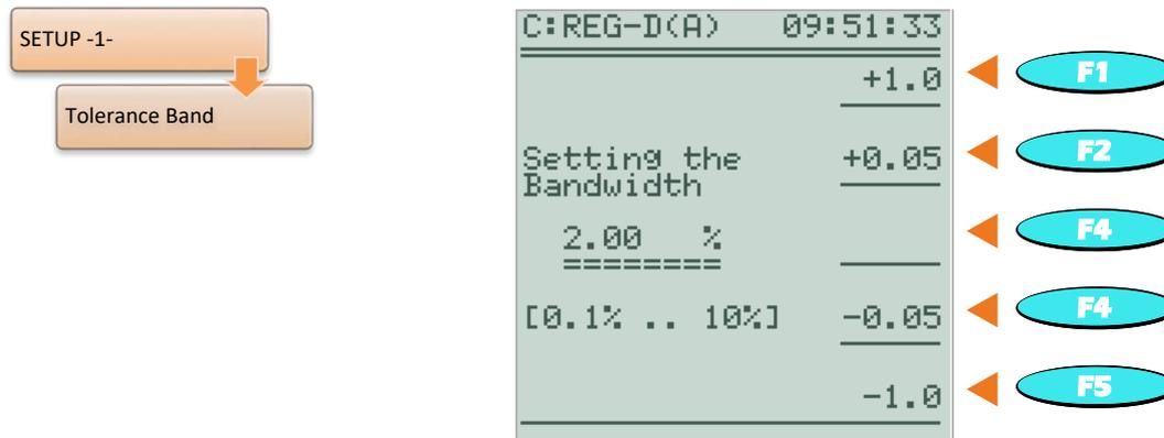
The current setpoint deviation  $X_w$  is the difference between the actual value  $X$  of the control value and the reference value  $W$  (setpoint value). The sign of the setpoint deviation can thus be positive or negative.
