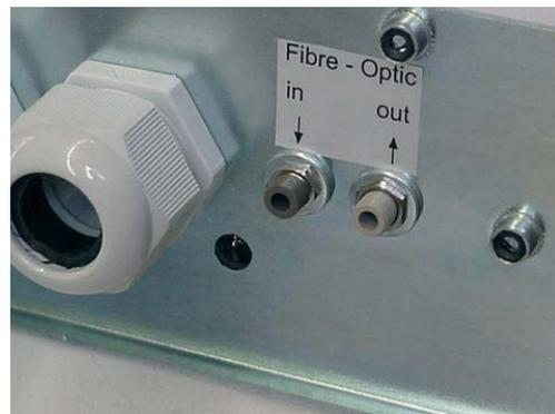
*Fibre optical connection (FSMA-connector, V13, V15)*
