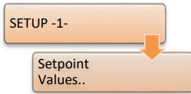
The Relay for Voltage Control & Transformer Monitoring REG-DA provides up to four setpoints. By default, the first setpoint value is selected. In the setup of setpoint values, the secondary value  $U_n$  is shown at the top of the setpoint display, below there is shown the primary value  $U_{LL}$  multiplied by the factor  $K_{nu}$ . The setpoint can be changed with the keys F1, F2, F4 and F5. Press Enter to confirm the entry.
