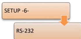
The COM1 interface is accessible as configuration or programming interface via a SUB-D connector on the front panel. Alternatively, the connection can be made via a mini USB cable (order code I1). By default the COM1 mode is ECL. In this mode, the regulator can be accessed using the software WinREG. BAUDRATE, PARITY and HANDSHAKE must match the settings of the connected end device (e.g. PC) to ensure trouble-free communication. The following communication parameters are recommended:
