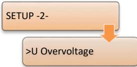
The overvoltage >U is a limit value which only influences regulation in special operating circumstances, and can be configured to a LED or an output relay, if necessary.
