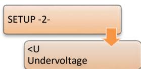
The undervoltage <U is a limit value, which only influences regulation in special operating circumstances, and can be configured to a LED or an output relay, if necessary.
