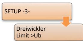
The limit >Ub is used to monitor the non-regulated voltage in an application with a three-winding transformer which has only one tap changer. Here, in general one of the two secondary voltages is selected for regulation. The other voltage can be monitored for exceeding an adjustable limit (>Ub). If the limit is reached, then up commands are blocked.
