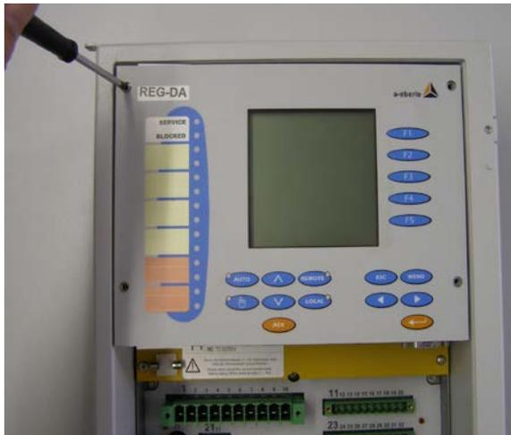
*Loosen the front panel of the REG-DA*
