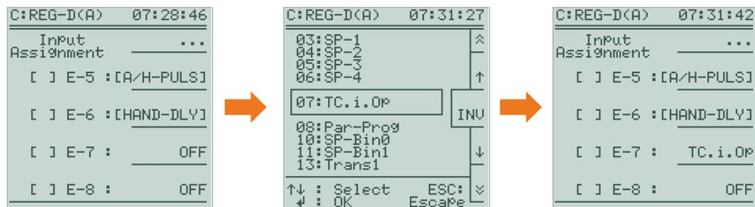
If an input function needs to be inverted, this can be accomplished in the function selection menu, using the F3 INV key. An inverted function is marked with a minus sign in front of the specific function.
