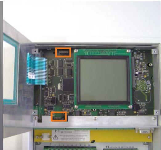
*Open front panel and position of the connectors (orange selection)*
