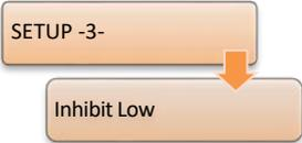
If the voltage goes below the limit for Inhibit low, the regulator shuts down. This means that automatic regulation is blocked and no more tap commands are issued. If the voltage exceeds the limit (plus hysteresis), the regulator operates in the usual manner.
