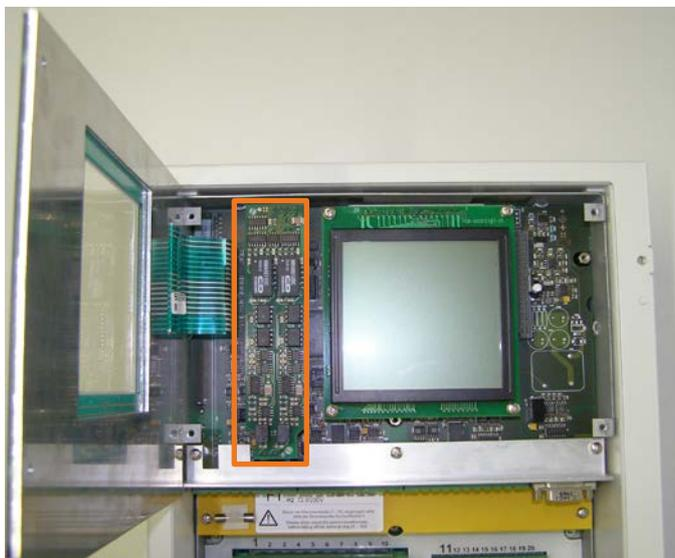
*Installed analog module*
